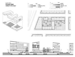
Figure 10: Diagram of mixed-use Folded Porous Block
